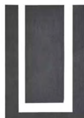
Fig : Molybdenum Crucible made by slip casting molybdenum powder of 2 to 3 \mu particle size fol-
