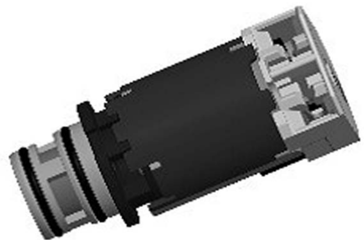
Dog Clutch with a Control Solenoid Valve
